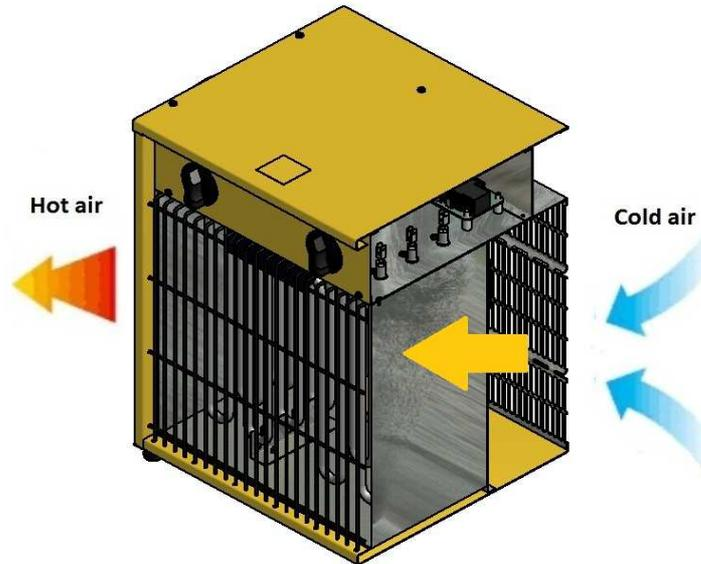
The device works on the principle of forced convection. The air flow is forced fan. Cold air is drawn in the back of the unit. Further, when flowing from the heater, it receives heat. The heated air is expelled in front of the heater. The device has a thermostat for the regulation of temperatures 5-35 °C. The unit area is equipped with thermal protection with reset. The unit features: ventilation, heating with half the power, heating at full power. The device has a cooling thermostat.
